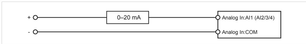
**Fig. 17 Analog Input – 2-wire Current Sensor**
